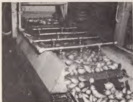
FIGURE 4.—Water is sprayed on sweetpotatoes going through a washer.
